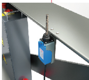
检修楼层盖板打开检测 Open detection when make overhauling over floor plate
