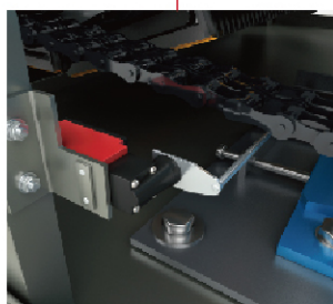
主驱动链断链保护装置 Protection device for chain scission of main drive chain
